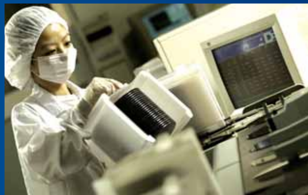
Wafers being gauged as part of the silicon reclaim process
