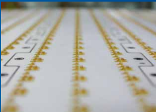
Close-up of the Probes on the SureTouch™ 300mm Full-Wafer One-Touch NAND Memory Probe Card
