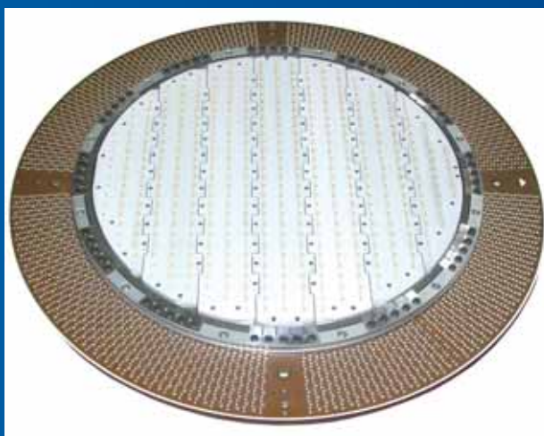
SureTouch™ 300mm Full-Wafer One-Touch Probe Card for Testing NAND Flash Memory Devices
