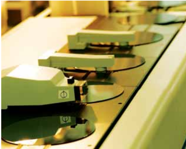
Wafer sorting line at our Tuas Silicon Reclaim Plant.
