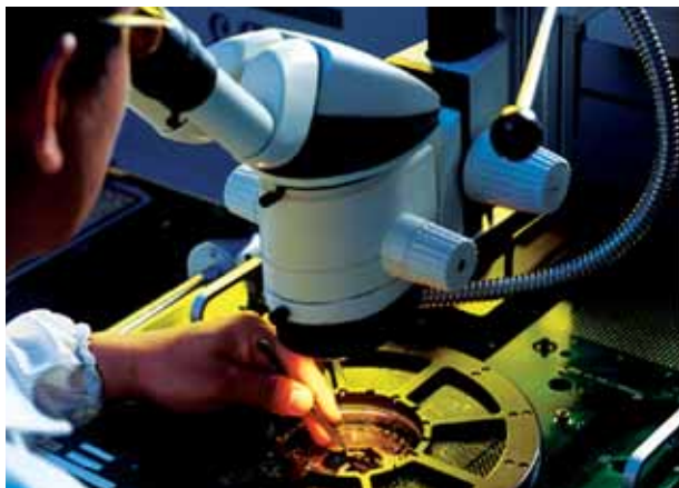
Operator inspecting a probe card
